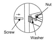
Turn the trolley upside-down and screw the swivel castors into the frame. Place the bumpers above the castors.
