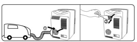
Dust and other dirt on the ventilator has a negative impact on cooling and heating capacity. Clean the ventilator regularly. A vacuum or brush can be used to clean dirt near the air outlets and intakes (dia. ① + ②).
