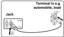
Plug one end of the **DC cable** into the DC terminal on the device ①, and the other end ② to a cigarette lighter jack.
