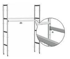
Insert 8 crossbars onto the connecting screws on side elements.
