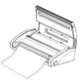
7. Then, place the open end of the trimmed vacuum sealing bag on the sealing strip of the unit, and not inside the vacuum chamber.
