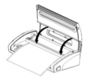
5. Pull the cutting mechanism down and lay it over the film roll.
