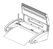
Move the blade from one end to another in order to accurately and cleanly cut off the vacuum bag.
