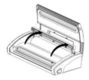
3. Raise the cutting mechanism and place the roll of film in the recess under the cover foreseen for this purpose.
