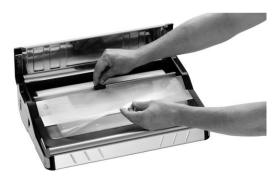
Place the cut vacuum bag on the sealing strip up to the marked edge, and not inside the vacuum chamber.
