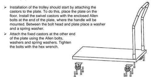
> Place the plate with wheels on one side, and firmly screw the handle to the plate with the Allen bolts, washers and spring washers.
