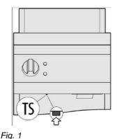
The appliance is equipped with a safety thermostat that interrupts power supply in the event of a failure.
