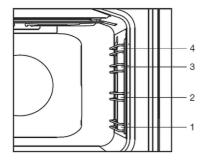
The thermal processing chamber of the appliance features several baking levels.
