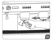
4. Fit the filled handle on the brewing group head and rotate it into the correct position.
