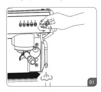
Set the steam nozzle over the drip tray and open the steam tap for a couple of seconds, to drain the water condensate.
