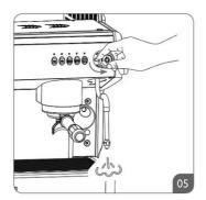
When the process is finished, direct the steam nozzle over the drip tray and open the steam tap for a couple of seconds to remove the milk left in the steam nozzle.
