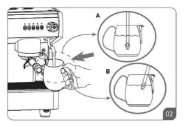
Immerse the steam nozzle in the milk container and make sure the nozzle is fully immersed.
