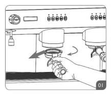
Rotate the handle out and remove it out of the brewing group.
