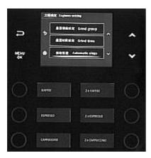
In the service menu use <sup>↑</sup> or V buttons, to select "Automatic slags" and confirm with OK.
