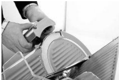
Fig. 3: Removal of the sharpener
