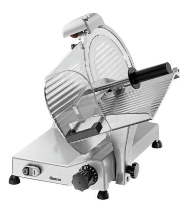
The design of the optimised slicing machine with its 220 mm blade stands out thanks to many technical features. The high-performance oblique slicer in 5 different sizes has a holder for remainders, a blade sharpener, a cutting guide and a two-fold blade guard as well as a solenoid switch to guarantee safety.
