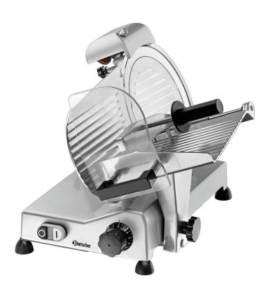
The design of the optimised slicing machine with its 220 mm blade stands out thanks to many technical features. The high-performance oblique slicer in 5 different sizes has a holder for remainders, a blade sharpener, a cutting guide and a two-fold blade guard as well as a solenoid switch to guarantee safety.
