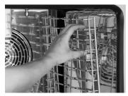
To facilitate the cleaning of the thermal processing chamber, remove guide rails from the appliance.
