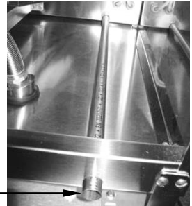
Dripping trough for condensed water
