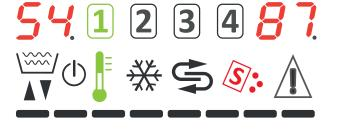
**IMPORTANT:** Before starting a regeneration cycle check if there is salt in the special container. When the **F8** indicator flashes on the display it means that the salt level in the bowl is low (only on machines equipped with the optional Water Softener).
