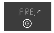
When in manual mode, at the moment doors are closed all settings return to zero and resets to the beginning of the setup process. If the time button is pressed the time indicator will be set to **000** and preheating will be stopped.
