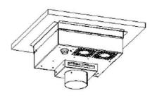
Clean the areas, where the selfadhesive strip is applied. Remove the excess of adhesive, cutting it off perpendicularly to the frame edge.  Fix the frame to the appliance and screw it back with the connection screws.
