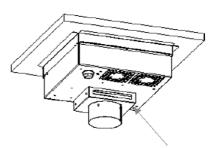
5. Connect a tube 100 mm in diameter to the fresh air supply duct.
